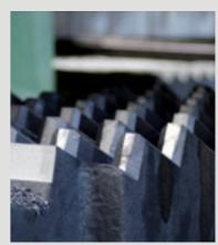
Cooling beds are crucial to the steel manufacturing process, carefully moving and cooling the hot steel after the rolling process. Since this is an integral part of a Steel Mill's manufacturing process, any mechanical problems or failures to the cooling bed will have huge consequences for the mill. The cooling bed and components therefore need to be manufactured to the highest quality standards and thoroughly tested before installation.
